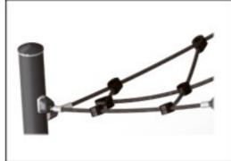
Rope loops of the seat are made of single braided 16 mm PES ropes. The polyester yarn is made from +95% post-consumer materials and is inductively melted onto each strand. PES has high strength with excellent resistance to abrasion and UV radiation. The rope loops are connected by nylon (PA6) connectors.
