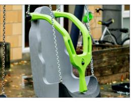
The Harness is made of molded recyclable polyethylene (PE) from 33% post-consumer materials. The Harness utilizes a stainless-steel torsion spring, which makes the Harness stay in all positions to secure easier user entry and exit. The harness lock is designed with a one-handed operation slider made from stainless steel.
