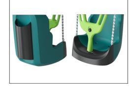
The front bumper has a solid polypropylene (PP) core with a softer outer layer of thermoplastic rubber (TPE) and an 8mm thick EPDM membrane rear bumper. The soft, shockabsorbent bumpers with nonslip surfaces make the swing seat highly safe for caretakers.
