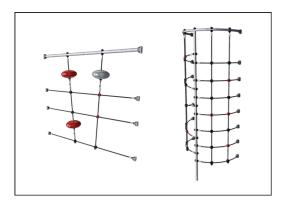
Ropes are made of UV-stabilized PES rope strands with inner steel cable reinforcement. The polyester wrapping is inductively melted onto each strand to ensure excellent wear and tear resistance.
