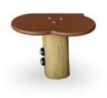
The steps are made of 21.5mm thick plywood which comes from alder and pine wood. Both sides are covered by two layers of phenolic film with anti-slip net pattern. All cutting edges are sealed with paint to ensure longivity.
