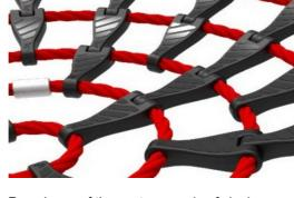
Rope loops of the seat are made of single braided 16 mm PES ropes. PES has high strength with excellent resistance to abrasion and UV radiation. The rope loops are connected by nylon (PA6) connectors.
