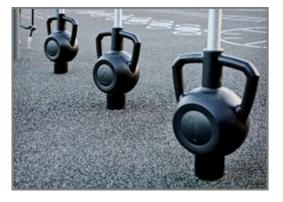
The tubes on which the magnetic bells move are ø40mm, made of grade AW 6082-T6 aluminium and have an anodized layer of  $20\mu$ m. The tube has a full steel core for structural integrity.
