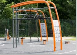
To ensure the integrity of the main frame, the orange coloured main posts are made of  $\emptyset$ 101.6 x 3mm steel posts, which are hot dip galvanised and powder coated Orange (RAL2010). The supportive posts receive the same surface treatment and are made of  $\emptyset$ 76.1 x 3.6mm steel tubes, powder coated grey (RAL7012).
