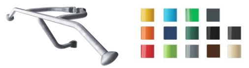
The frame of the leg lift is made from Ø38 x 2mm HDG steel tube. The support plates are made from 15mm Ekogrip®, a 15 mm PE plate with a 3 mm top-layer of thermoplastic rubber with non-skid effect. The arm supports are 110 x 195mm, 580mm apart, and 1315mm above ground. The back support is 335 x 500mm. The opening in the back is 30 x 350mm. The pull up bar is made from Ø32 mm HDG steel bar. The bar is 1080mm wide and 2300mm above ground
