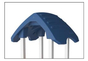
The large hollow components are made of 100% recyclable PE. The roof displayed is moulded in one piece with minimum 5,5mm wall thickness to ensure high durability in all climates around the world.
