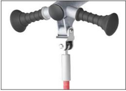
The two angled top handles are made of a moulded PP insert with an outer soft layer of TPV rubber. The handle is attached to the pipe with a galvanised steel inlay to ensure strength and durability.
