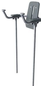
The frame of the leg lift is made from Ø38 x 2mm HDG steel tube. The support plates are made from 15mm Ekogrip®, a 15 mm PE plate with a 3 mm top-layer of thermoplastic rubber with non-skid effect. The arm supports are 110 x 195mm, 580mm apart, and 1315mm above ground. The back support is 335 x 500mm. The opening in the back is 30 x 350mm.
