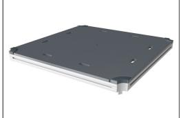
All decks are supported by unique designed low-carbon aluminum profiles with multiple attachment options. The grey colored molded decks are made of 75% post-consumer waste PP material with a non-skid pattern and texture surface.
