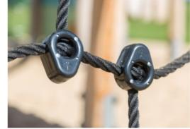
Nets and ropes are made of UV-stabilised PA with inner steel cable reinforcement. The rope is induction treated to create a strong connection between steel and rope, which leads to durable weather resistance.
