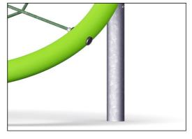
The rope is fixed to the large steel pipe by a unique KOMPAN designed tightening solution. It consists of inner and outer nylon (PA6) bushings that guides the rope to an outside threaded aluminum part that tighten the rope.
