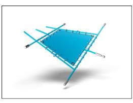
Corocord membranes consist of friction-proof rubberized material of conveyor belt quality with excellent UV resistance. Tested and compliant with REACH requirements for PAH. Embedded is a four-layered armouring made of woven polyester. The armouring and the two surface layers result in a total thickness of 8 mm.
