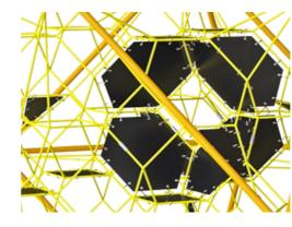
Corocord membranes consist of friction-proof rubberized material of conveyor belt quality with excellent UV resistance. Tested and compliant with REACH requirements for PAH. Embedded is a four-layered armouring made of woven polyester. The armouring and the two surface layers result in a total thickness of 7.5 mm.
