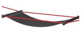
Corocord membranes consist of friction-proof rubberized material of conveyor belt quality with excellent UV resistance. Tested and compliant with REACH requirements for PAH. Embedded is a four-layered armoring made of woven polyester. The armoring and the two surface layers result in a total thickness of 7.5 mm.
