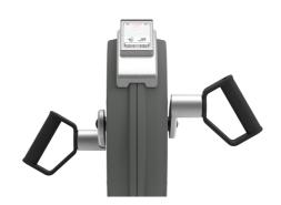
The Q-factor of the arm bike is 175mm, the crank is made of 18 mm stainless steel and connects the pedal arms which are casted stainless steel (grade 304) parts. The length of the pedal arms is 170mm and the pedals are connected with standard bike fittings.
