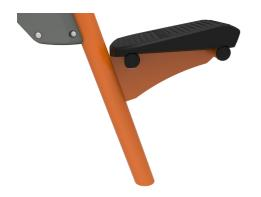
The seat is made of a Polyurethane Rubber and has a steel insert plate which connects it to the steel frame. The seat is positioned under a 12 degree angle, accommodating seating heights from 550-620mm.
