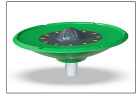
The outer ring of the Spinner Disc base is made of recyclable LDPE. The ring is moulded in one piece with integrated metal thread bushings and water drain holes to ensure high durability in all climates around the world.
