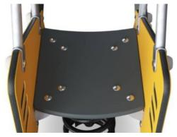
Seat is made of Ekogrip™ panel that consist of a 15mm thick PE base with 3 mm top-layer of soft rubber with a non-skid effect.
