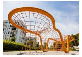
The steel surface of these bended steel pipes are wet painted with one basic layer and one top layer of lead free colour material. The paint has excellent corrosion resistance and can be easily maintained.
