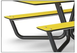
All boards are made of High Pressure Laminate HPL with a thickness of 17.8mm according to EN 438-6 and has a nonskid surface texture. The multilayer construction makes the boards durable and suitable for outdoor use with a high UV stability and high resistance to impacts, scratches, fire, water and humidity.
