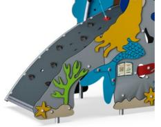
Curved climbing wall is made of Ekogrip® panel that consist of a 15mm thick PE base with 3 mm top-layer of soft rubber with a non-skid effect.
