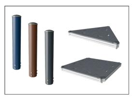
The main posts are made of high quality pregalvanized steel with powder coated top finish. Post tops are closed with caps of UV stabilized nylon (PA6). The grey colored molded decks are made of 75% post-consumer waste PP material with a non-skid pattern and texture surface. All decks are supported by unique designed low-carbon aluminum profiles with multiple attachment options.
