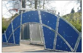
The goal measures ~140cm in depth and ~330cm in width with all posts made of galvanized steel with a hot dip galvanized surface treatment. The front frame is made with Ø48 tubing, and the backside of the goal uses 10 tubes with a diameter of ø38.
