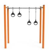
**Installation Information** Max. fall height 200 cm Safety surfacing area 67.7 m<sup>2</sup> Total installation time 14.3 1.40 m<sup>3</sup> Excavation volume Concrete volume 0.84 m<sup>3</sup> Footing depth (standard) 90 cm Shipment weight 863 kg Anchoring options In-ground Surface
