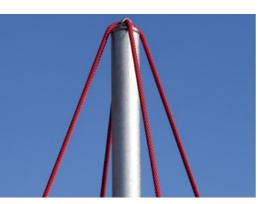
In the centre of the net is the mast, made of high quality seamless steel. The structure of the mast as an oscillating support is statically favourable and equalizes the oscillations in the net. The masts are hot dip galvanised as standard, with the design option of additional powder coating.
