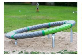
The Supernova is a unique carousel with no centre point placed in an angle of 10° which makes it turn when children walks the ring. The outside ring diameter is 208cm and the upper point is 60cm above ground level.
