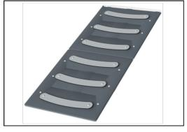
The ramp deck is made of High Pressure Laminate HPL with a thickness 17.8mm and non skid surface texture according to EN 438-6. KOMPAN HPL has high wearing strength to ensure long lifetime in all climates.
