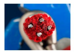
Corocord 16mm ropes are special 'Hercules'type with galvanised four-stranded steel wires and a steel wire core. Each strand is tightly wrapped with PES yarn, which is melted onto each individual strand. The ropes are highly wear-and vandalism-resistant and can be replaced at site if needed. English version
