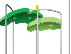
**Installation Information** Max. fall height 204 cm Safety surfacing area 65.6 m<sup>2</sup> Total installation time 36.0 Excavation volume 1.34 m<sup>3</sup> Concrete volume  $0.74 \text{ m}^3$ Footing depth (standard) 60 cm Shipment weight 1,181 kg Anchoring options Surface In-ground
