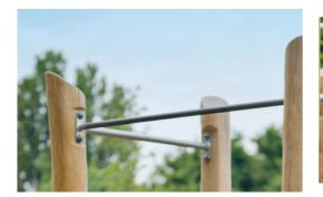
All bars intended for pull ups are made of solid, ø32mm x 138 m, hot dip galvanised, S235JR steel bars. This diameter gives the right grip for everyone.
