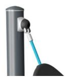
Unique KOMPAN swivel suspensions allowing for both swinging and rocking movement of the hammock. The inside housing is made of stainless steel and both the bushing and bearing rod of brass alloy. The outside cover is made of soft TPV rubber and the entire swivel is attached to the steel post by an aluminum connector.
