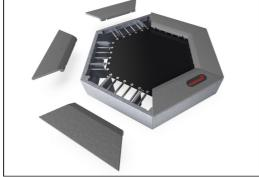
As a unique feature the SBR tiles can be removed for cleaning and service. By loosen six screws the SBR tile can be lifted up to open and gain access to the springs (see instruction on KOMPAN Master).
