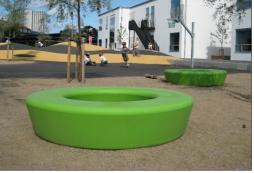
The Loops can be anchored to the ground by filling them with water or sand using integrated plugs. Alternatively, they can be secured using surface or ground brackets.
