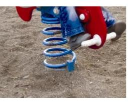
KOMPAN's springs are manufactured from highquality spring steel. The springs are cleaned by phosphating before being painted with epoxy primer and polyester powder coating. The springs are fixed by unique anti-pinch fittings for maximum safety and longevity.
