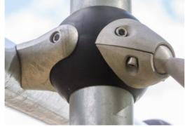
The unique designed GALAXY connection ball is produced with an inner circular core of aluminium surrounded by a shell of hard PP with an outer layer of soft TPV rubber. Flexible lead-free aluminium connectors allow for installation in variable angles.
