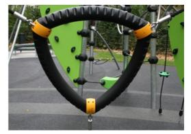
GALAXY climbing triangle with an outer soft layer of PUR and corner brackets of moulded nylon (PA6). The core consists of a powder-coated welded steel frame with integrated corner suspension points. Larger triangles are closed with an 18mm thick Ekogrip® panel that has a top layer of rubber with a non-skid effect.
