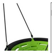
The shell seat is made of 100% recyclable polyethylene (PE) and rotomoulded in one piece. The seat is designed with large outer openings for handholds and middle holes for drainage of water and dirt. The four ropes are attached with hot dip galvanised steel brackets to ensure durability for many years.
