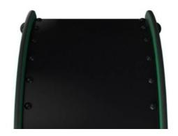
Membranes consist of friction-proof rubberised material of conveyor belt quality with excellent UV resistance which is then embedded is a four-layered armouring made of woven polyester. The armouring and the two surface layers result in a total thickness of 9 mm.
