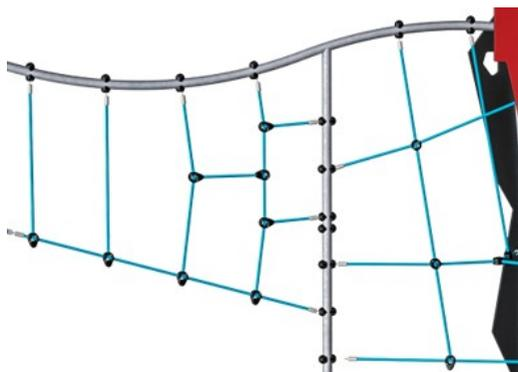
Ropes are made of UV-stabilized PP rope strands with inner steel cable reinforcement. Horizontal ropes are PUR coated to obtain good wear and tear resistance.
