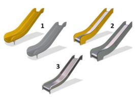
Slides are available in three different materials: moulded on piece PE slides made from 33% post-consumer materials, Combined EcoCore ™ sides and stainless steel slide bed t=2mm. Full stainless steel AISI304 t=2mm. The main posts are equipped with hot dip galvanised steel footings. The steel footings elevates the posts 20mm from ground level to avoid contact with surfacing material.
