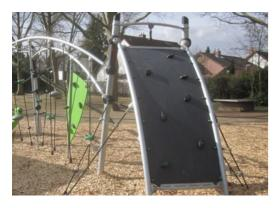
The curved climbing wall is made of a steel frame supported Ekogrip® panel with unique designed climbing cleats. The Ekogrip® panel consist of a 15mm thick PE base with 3 mm top-layer of rubber with a non-skid effect.
