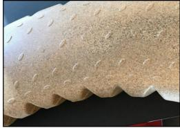
The sand colored variant is made of rotomolded stone mixed PE made from 33% post consumer materials with a non skid surface texture. Minor differences in the stone mix visuality of the material are to be expected.
