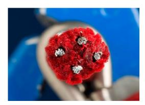
Corocord 16mm ropes of UV-stabilized PES rope strands with inner steel cable reinforcement. The polyester yarn is made from +95% post-consumer materials and is inductively melted onto each strand. The ropes are highly wear-and vandalism-resistant and can be replaced at site if needed.
