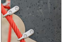
Corocord membranes consist of friction-proof rubberized material of conveyor belt quality with excellent UV resistance. Tested and compliant with REACH requirements for PAH. Embedded is a four-layered armoring made of woven polyester. The armoring and the two surface layers result in a total thickness of 7.5 mm.
