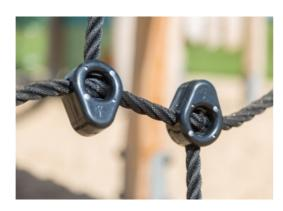
Nets and ropes are made of UV-stabilized PA with inner steel cable reinforcement. The rope is induction treated in order to create a strong connection between steel and rope which leads to good wear resistance. The Robinia wood can be supplied as untreated raw wood or painted with a brown colored transparent pigment that maintains the golden wood color of the wood.
