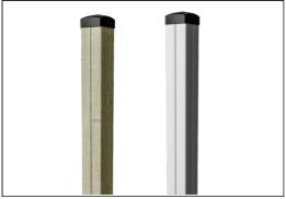
The main tower posts are available in two types of material: European pine wood posts, pressure impregnated Class 3 with Tanalith E3475 according to EN335 (Equivalent to NTR Class AB). Aluminum post t=2mm with anodized surface treatment. Base material FN AW-6060 T66.
