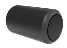
The rotating rollers are Ø 110mm and made from PUR (Polyurethane Rubber, compact foam). The rollers have a steel insert that is electro galvanized. They provide support and ensure a comfortable position.
