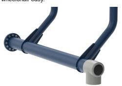
The input shaft is Ø101,3 x 2,9mm S355 Hot Dip Galvanized and Powder-coated steel. The bearing house is Caste Aluminum (EN AB-44100 / EN AB-AISi12(a)) with self-aligning sealed ball bearings. An extremely strong and durable construction
