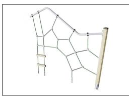
Corocord ropes of UV-stabilized PES rope strands with inner steel cable reinforcement. The polyester yarn is made from +95% postconsumer materials and is inductively melted onto each strand. PES has high strength with excellent resistance to abrasion and UV radiation. The rope loops are assembled by aluminum connectors.
