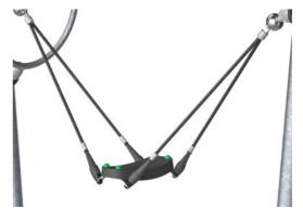
GALAXY ropes has six-stranded steel wires and a steel wire core. Each strand is tightly wrapped with PES yarn, which is melted onto each individual strand. The PES yarn is made of +95% Post-consumer materials and is inductively melted onto each strand to obtain excellent wear and tear resistance.
